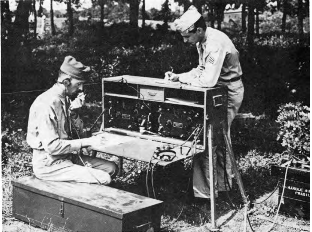
THE SCR-177. Receiving position showing the BC 314-C and BC 312-C receivers.
