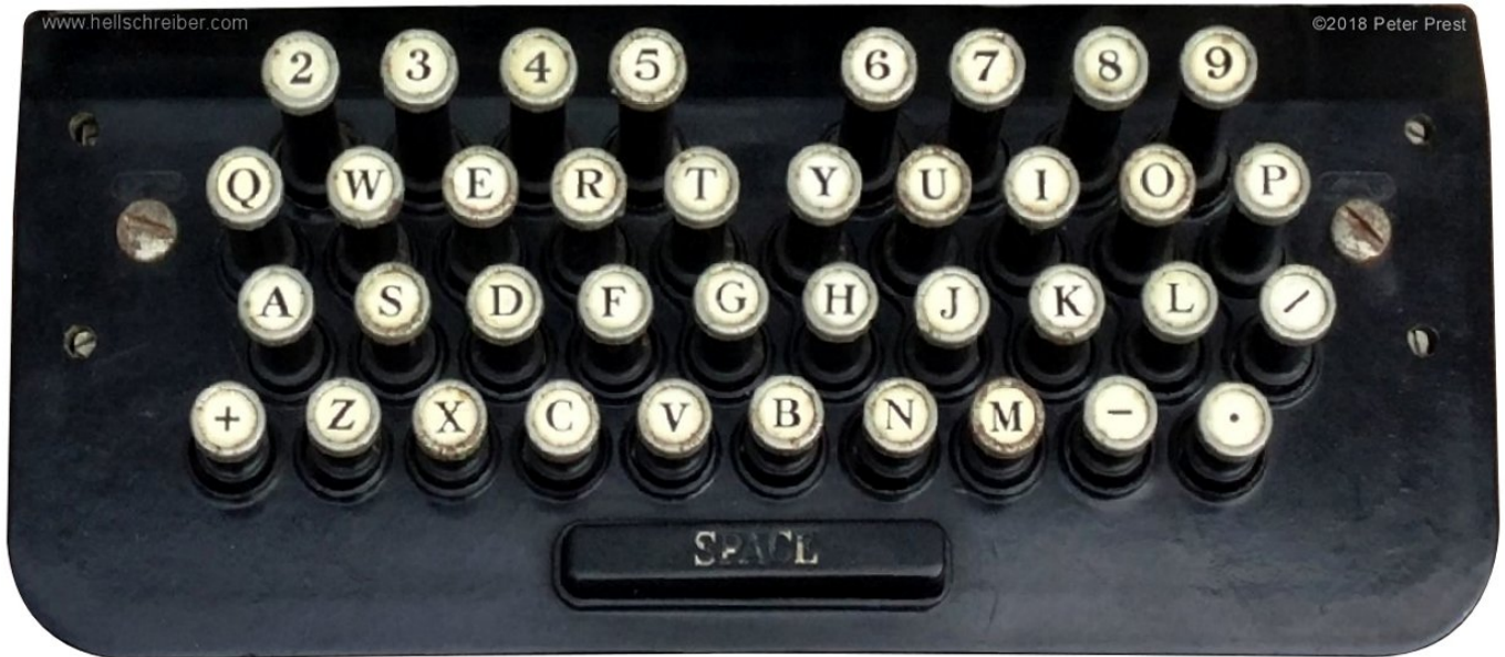
Figure 5: Four-row keyboard layout of the Telewriter machine (original unedited photo: ©2018 Peter Prest)
