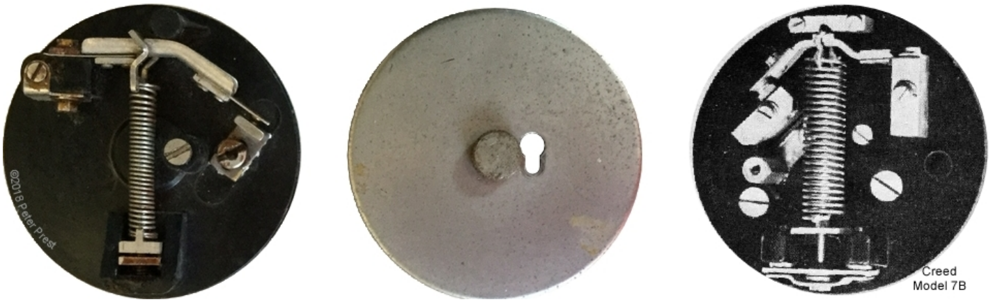
Figure 17: The centrifugal governor with its cover - for comparison, the governor of a 1930s Creed 7B teleprinter (unedited original photo: ©2018 Peter Prest; source photo Creed governor: ref. E)
