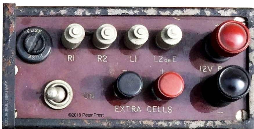
Figure 26: Panel with main switch, fuse, and terminals for phone line & batteries (original unedited photo: ©2018 Peter Prest)
