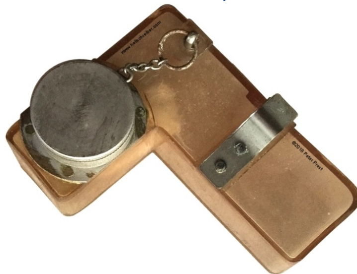
Figure 29: The water container, with the wick holder cap screwed on (original unedited photos: ©2018 Peter Prest; used with permission)
