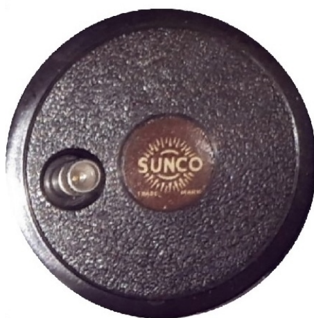
Fig. 27: Top of the "incoming call" buzzer, made by Sun Electrical Co. Ltd., and 1918 SunCo advertising
