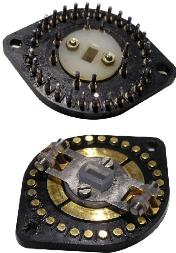
Figure 11: Painton & Co. Ltd. "Winkler" switch wafer and 1952 advertising
