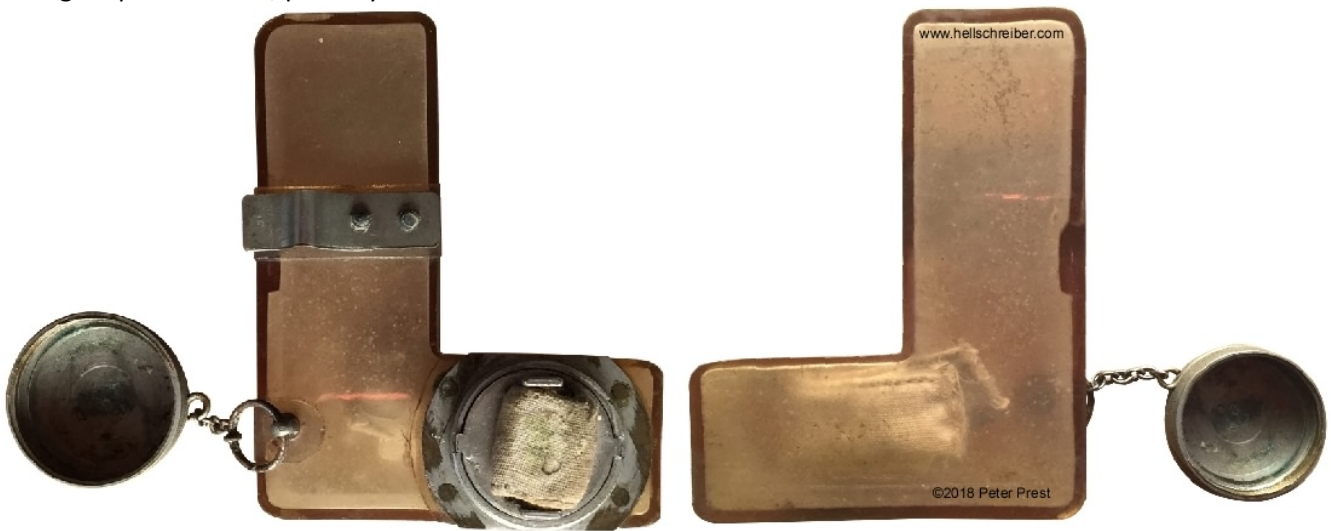
Fig. 28: Top & bottom of the water container with screw cap - note wick holder and the coarse cloth wick
