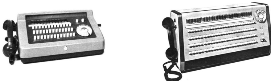
Figure 6: Standby Manual Exchanges – 16-Line (left) and 25-Line (right)
