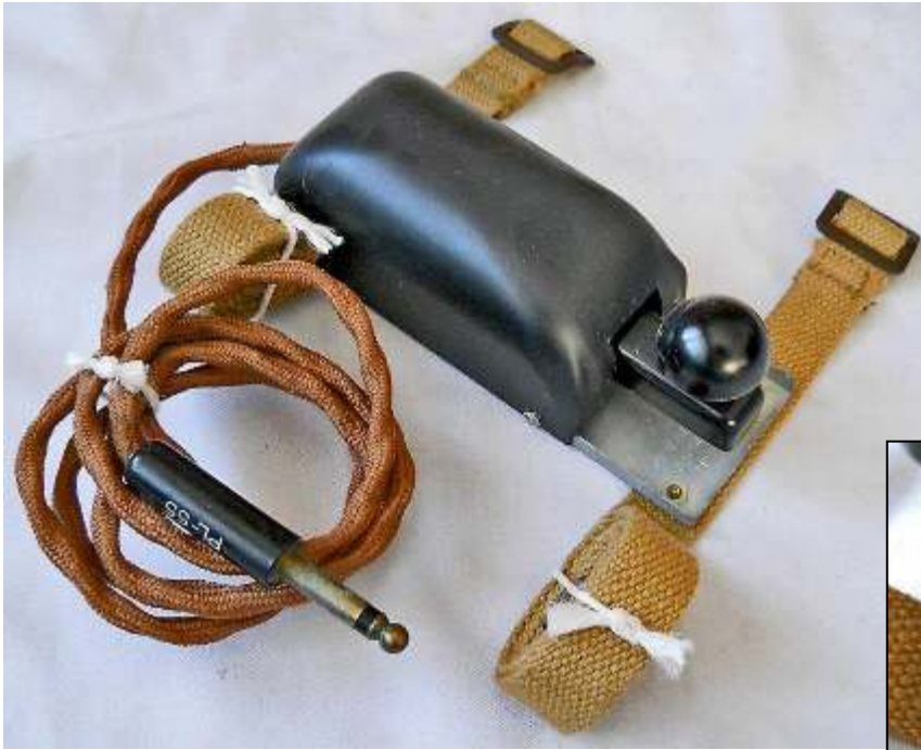
Key and Plug Assembly Cdn No. 9 Type 2 had a matt black rounded protective cover of pressed steel and a type PL-55 plug (left).
