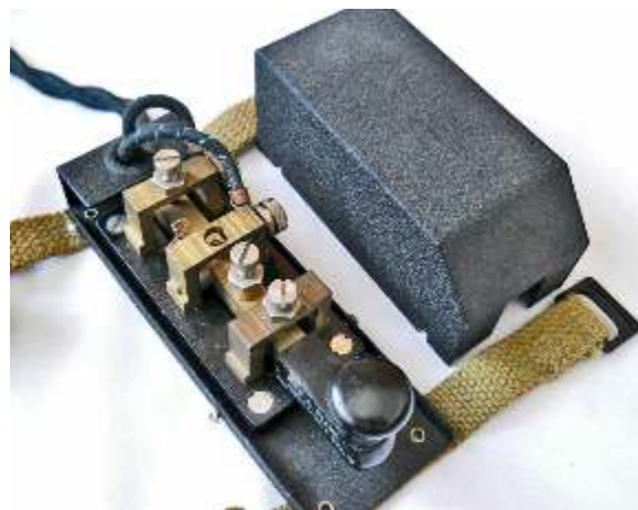
Key and Plug Assembly No. 9 ver. 9.1 was produced in the U.S.A. by J.H. Bunnell. Most significant differences to the British parent assembly were a type PL-55 plug and a smaller key knob.
