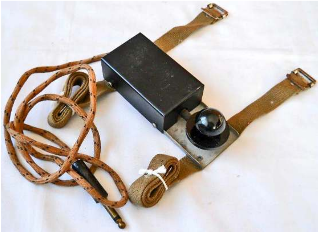
Key and Plug Assembly No. 9 ver. 10.2 was issued with Wireless Set No. 19 Mk.II produced in the U.S.A. It was nearly identical to ver. 10.1. Note the use of an American type PL-55 jack plug.
