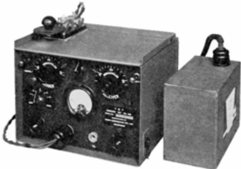
Key and Plug Assembly No. 2B (Aust) attached in a slide fitted on the inside of the front panel protection lid of Wireless Set No. 208 (above).
