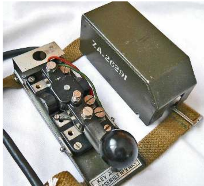
Front view of Key and Plug Assembly No. 9 Mk.1/1 (above) and with protective cover removed (right). Note that all the brass parts of the Key W.T. 8 Amp No. 2 Mk.III and the plug were plated.
