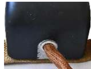
The rear of the metal plate had only one opening in the centre and a simplified lead tension restraint.
