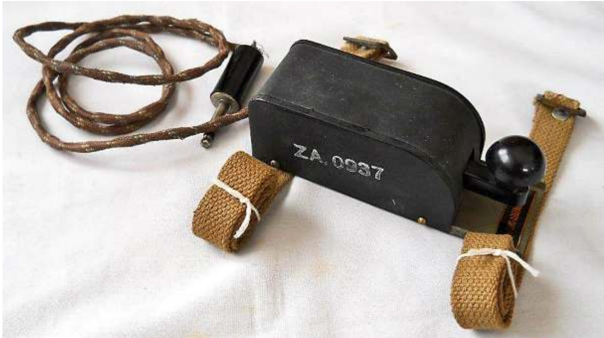
Key and Plug Assembly No. 9 ver. 3.3 was principally similar to ver. 3.2, but having a rounded protective cover.
