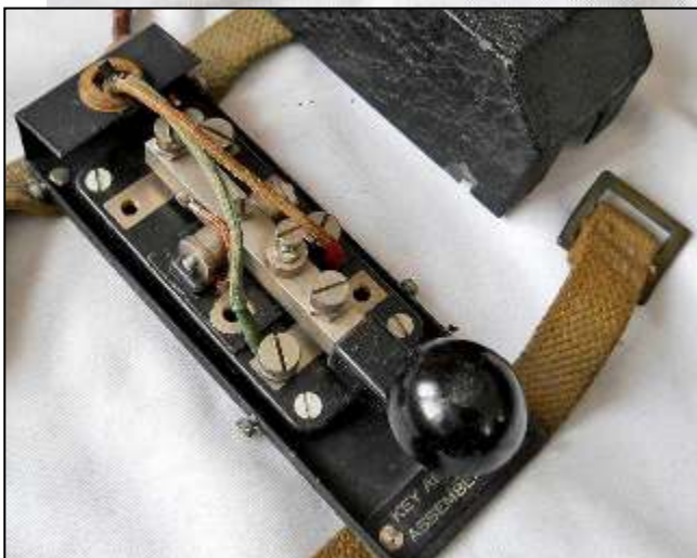
Key and Plug Assembly No. 9 ver. 1 (top of page), and without protective cover (above). The Morse key fitted in the assembly on the picture was a Key W.T. 8 Amp No. 2 Mk.II with a brass key lever.
