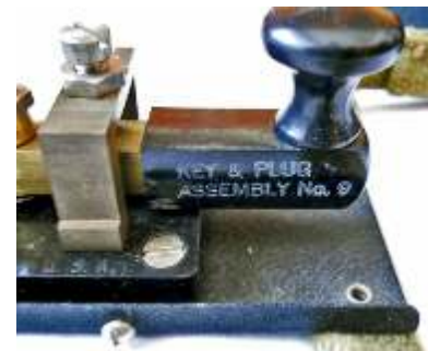
The assembly designation was ink stamped on the Morse key lever insulation sleeve (above). Note the smaller and differently shaped key knob.
