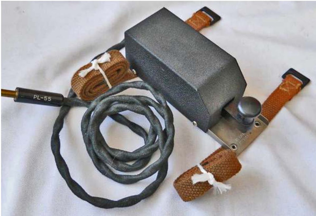
Key and Plug Assembly No. 9 ver. 9.2 was produced in the U.S.A. by J.H. Bunnell. It was a variant of ver. 9.1 with a plated assembly base plate and its designation stamped into this plate.
