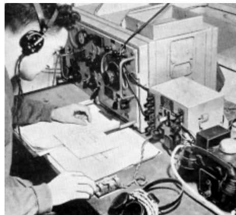
Wireless Remote Control Unit C allowed remote operation of Wireless Set No. 12 or No. 33. A Key and Plug Assembly No. 2B was issued with this unit (above).
