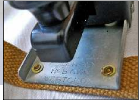
Front view of the No. 9 Type 2 assembly showing a slightly different key lever insulation sleeve (below).
