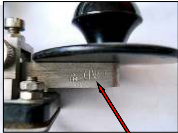
Detail view of key lever showing Australian markings 'D' 'broad arrow' D'.
