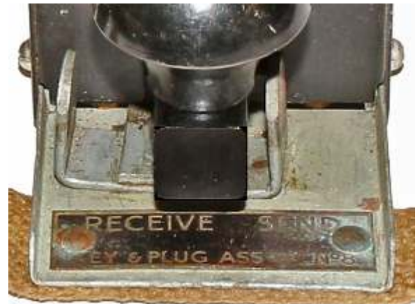
Detail view of send-receive switch lever under the key lever showing a slightly different designation plate reading ASS BLY (above).
