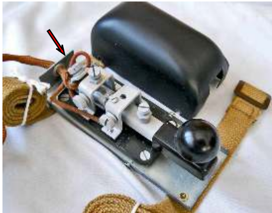
Key and Plug Assembly Cdn No. 9 Type 2 with its protective cover opened showing a Key W.T. 8 Amp No. C3 with two bridges of pressed steel construction (left).
