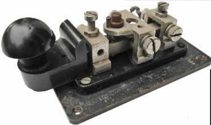
Surviving Key and Plug Assembly No. 6 with Key W.T. 8 Amp No. 3 mounted on a brass base plate. Note the insulating sleeve over the key lever.
