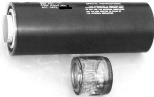
A three-stage image intensifier made by English Electric, below it is a wartime Tabby tube for comparison
