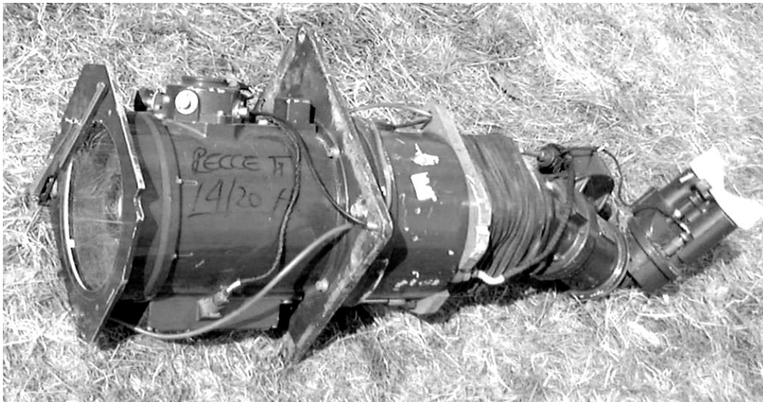
Sight, Periscope, AV, Image Intensified, L3A1
