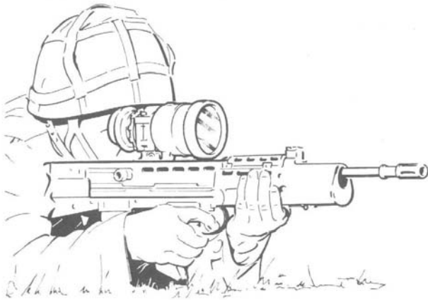
Weaponsight, Image Intensified, L6A1 on Rifle, 5.56mm, L85A1
