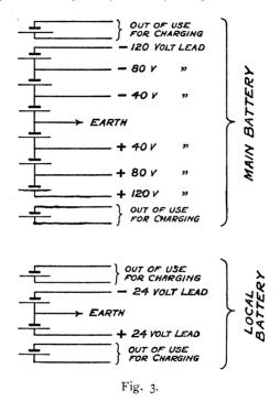
This arrangement fulfils condition (5), since only 64 cells or 44.4 per cent. in excess of working requirements are necessary.
