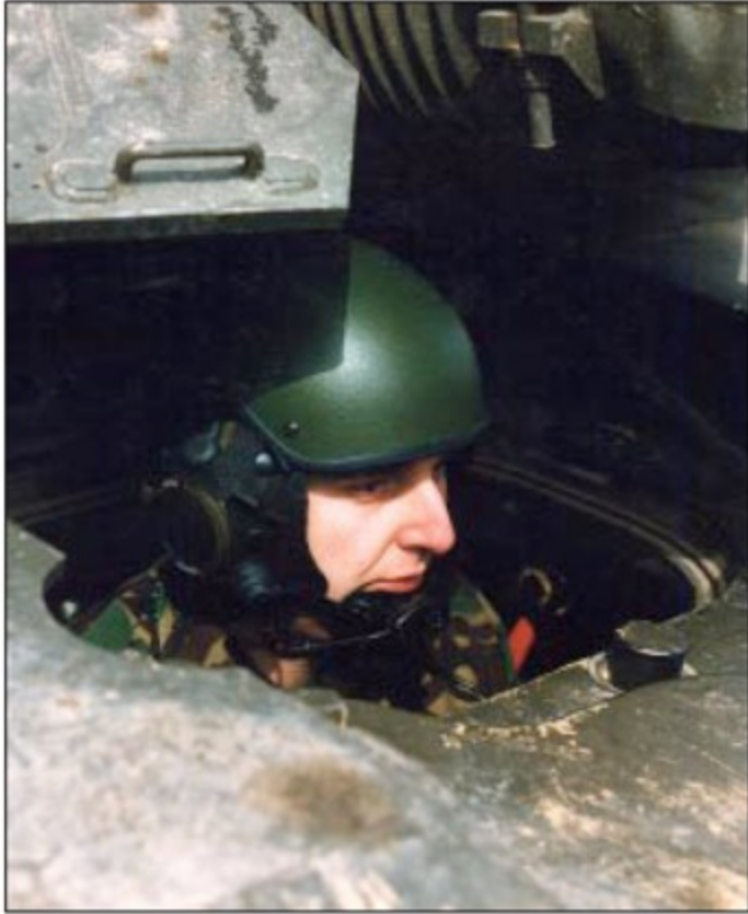
The hard helmet shell can be provided with a range of bump/ballistic protection levels.
