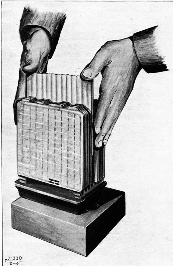
Fig. 6—Correct method of inserting a separator
