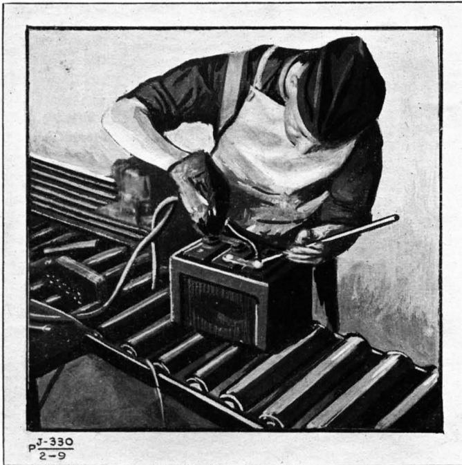
Fig. 9—Lead-burning an inter-cell connector
