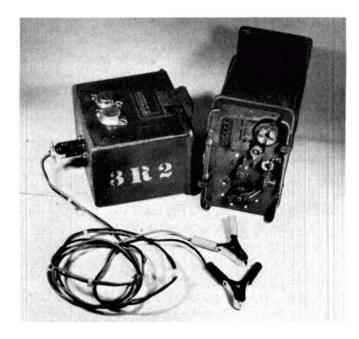
fig. 6. The complete radio set, shown with power supply and cable, measures 3  $\times$  4.75  $\times$  10.34 inches (7.62  $\times$  12.07  $\times$  26.26 cm).
