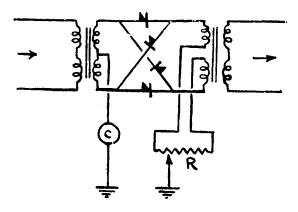
Fig. 7. Carrier leak potentiometer.
