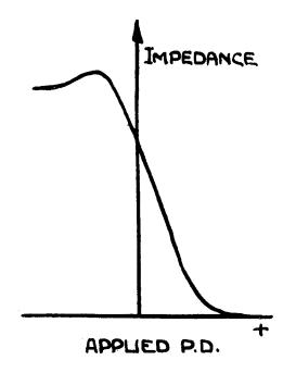
Fig. 6. Characteristic of copper oxide rectifier.
