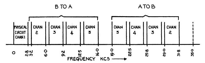
$F^{14}$ . 3. Diagram of channels in frequency spectrum of Army 1+4 carrier system working two-wire.
