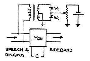
Fig. 8. Automatic limiter circuit for 500 c/s signalling tone.
