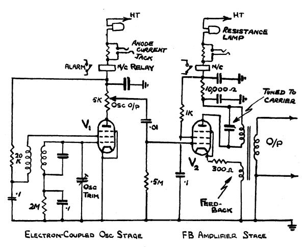
Fig. 9. Channel oscillator.
