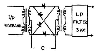
Fig. 5. Skeleton circuit showing principles of demodulation.
