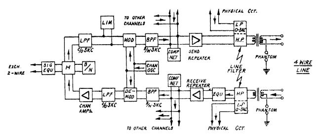
Fig. 10. Block schematic diagram of four-wire terminal.
