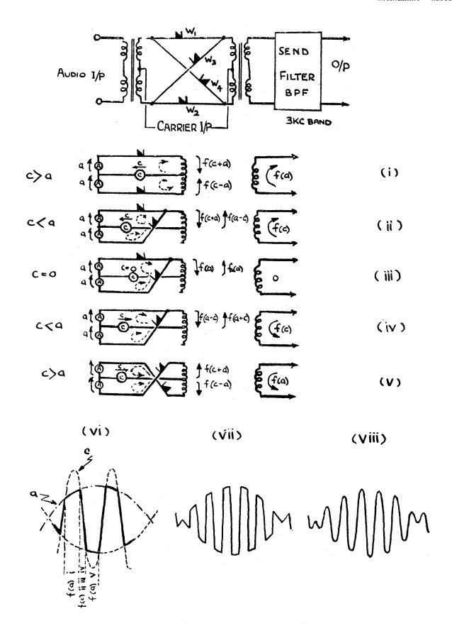
Fig. 4. Action of rectifiers in modulation.
