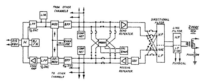
Fig. 11. Block schematic diagram of two-wire terminal.
