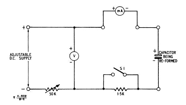
Fig 1 - Simple re-forming circuit
