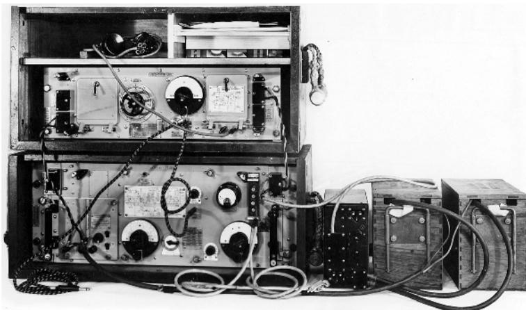
*Wavemeter Class B No. 1* is comprised of Naval type Wavemeter G61 and Oscillator G35. It is powered by Wireless Set No. 11 Supply Unit Low Power No. 1
