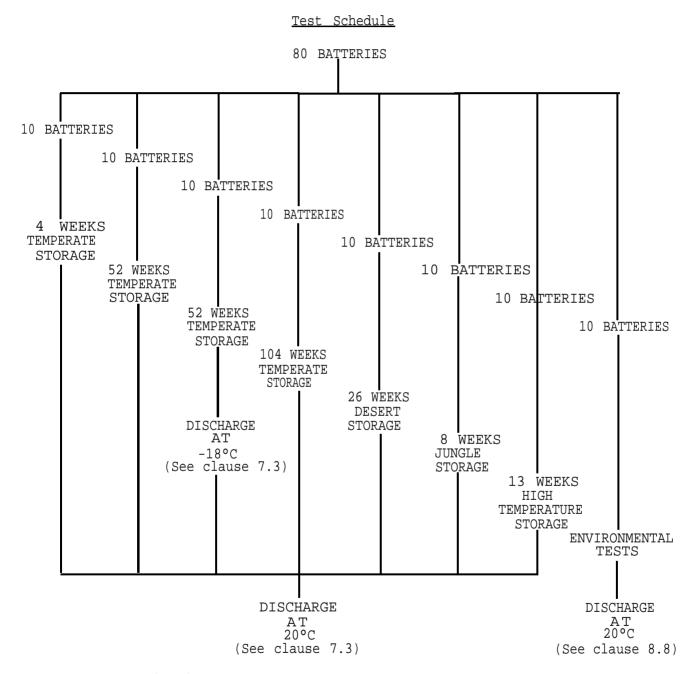
At least 8 batteries in any Sub-group of 10 and at least 71 batteries of the total of 80 batteries tested shall give not less than the minimum service output specified in clause 7.2, or clause 8.8.
