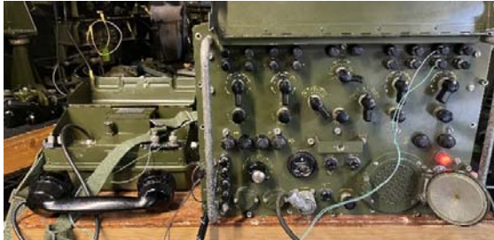
Figure 8. Testing a channel on the CST 1+4 No. 3 with a field telephone – telephone set J
