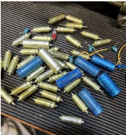
Figure 5. A selection of the faulty electrolytic capacitors replaced
