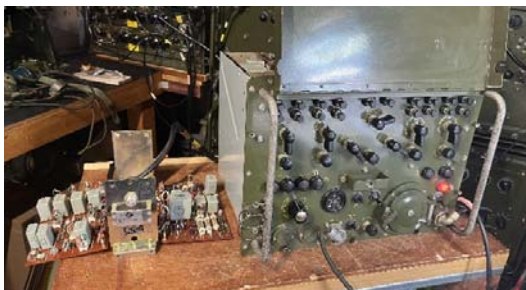
Figure 3. The carrier set telephone removed from its case and repairs/testing underway. Note the PCB is removed from the unit and checked externally with the aid of the extension cable supplied with the unit
