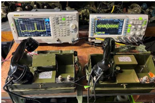
Figure 11. The test setup with two telephone set J's, and monitoring the frequency spectrum/baseband with the spectrum analyser and additionally with the oscilloscope
