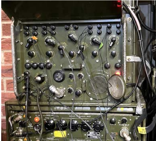
Figure 14. Final settings for the testing with the radio relay terminal. Note the meter selector switch is set at REC PILOT, thus monitors (and checks) the REC LINE signal in for the correct level (meter indicator central/in the white zone)
