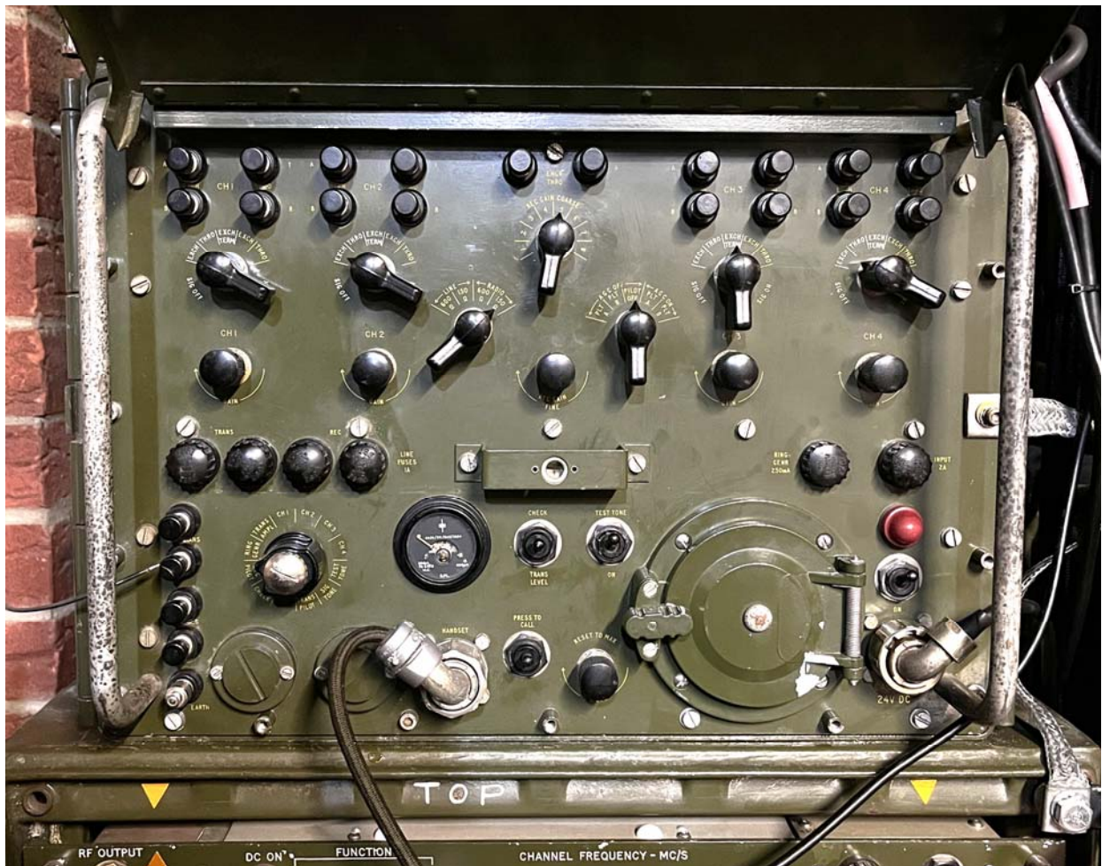
Figure 6. Front panel layout of the carrier set telephone showing the controls and the TMS unit/meter
